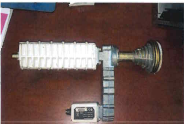
Anatel BUB Transmitter - Faulty
